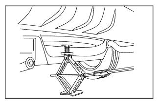
6. Lower the jack by turning the folding wrench counterclockwise. Keep lowering the jack until the spare tire is resting on the folding wrench.
